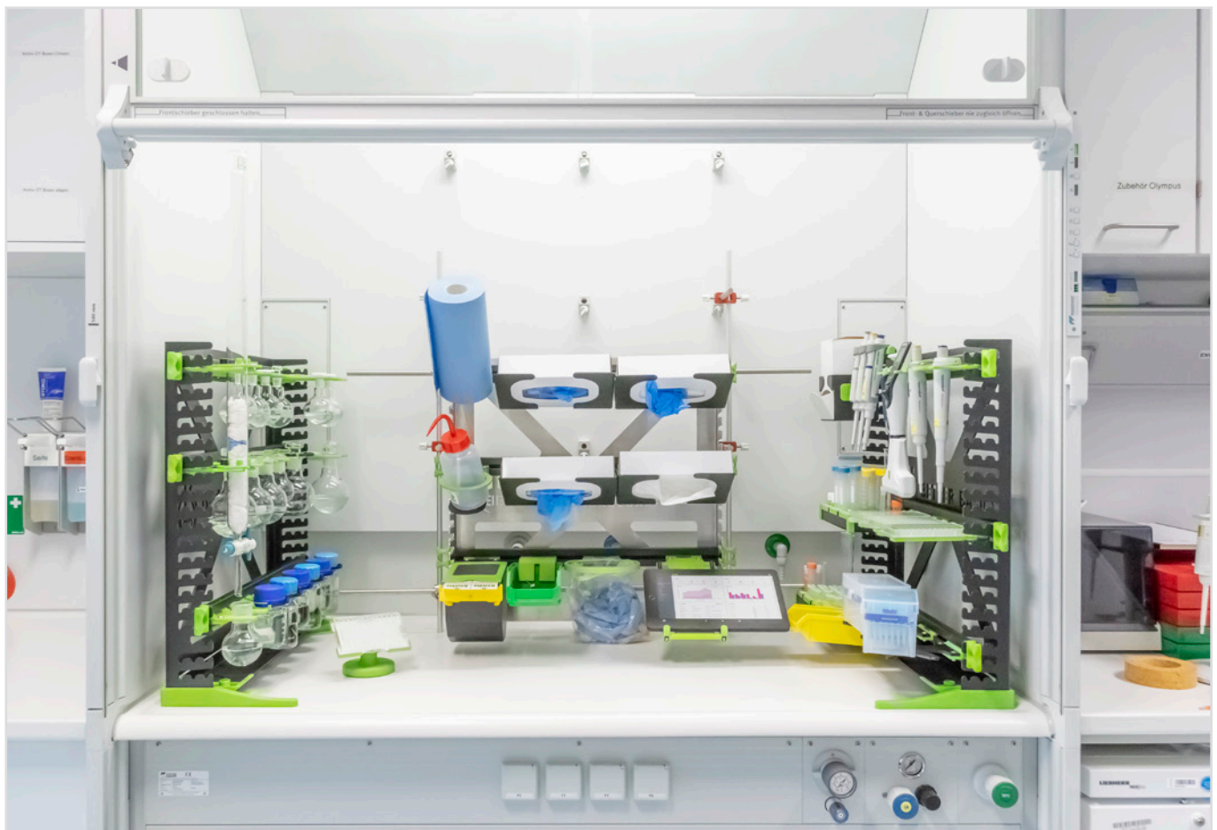
Two SmartRack® and one SmartFrame MB 001 with a SmartStand in a Wesemann fume hood
