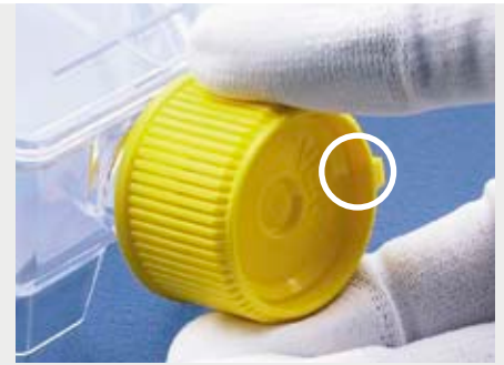
VENT position at 3 o'clock = gas tight
